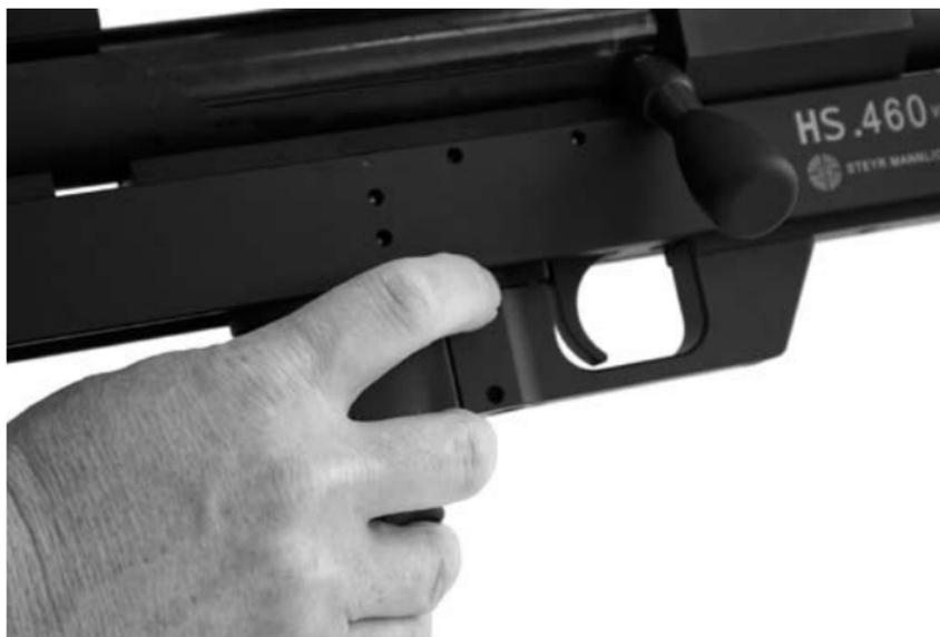
Make the rifle safe by sliding back the safety catch lever with the right index finger – red dot is NOT visible.
