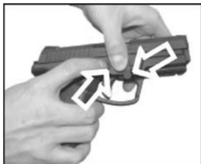
Lift closing spring and remove slide.
