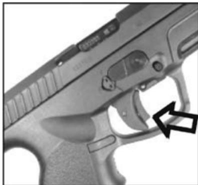
The loaded chamber indicator visibly and tangibly protrudes from the rear of the slide (optional).
