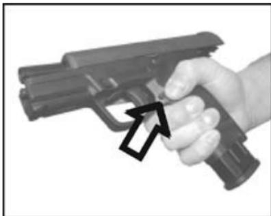
Check to make sure that no cartridge is lodged in the barrel.
