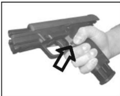
Check to make sure that no cartridge is lodged in the barrel.
