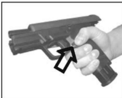
Retract slide to eject the cartridge lodged in the barrel.
