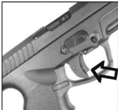
The loaded chamber indicator is visible and can be felt with the hand/finger.
