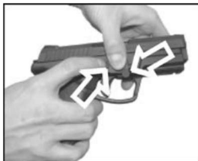
Lift closing spring and remove slide.
