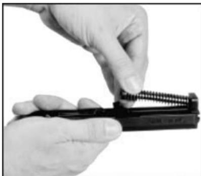
Hold barrel on bolt lock, lift and remove from slide by pulling it up and back.
